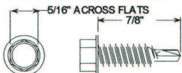
#14-7/8" Mill Point Hex Washer Head Metal to Metal (Max. 18 ga. panel )
