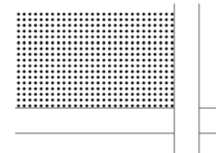
Pattern 98R216L 0.098" diameter holes, 0.216" lineal centers / no border / 16.2% open area (formerly pattern D)
