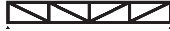
Bottom Chord-Bearing Floor Or Roof Truss (can design with a chase as well)
