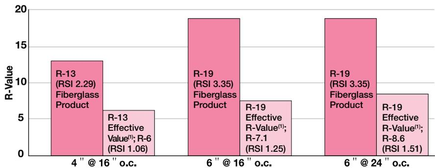
(1) Effective R-value (RSI) calculations based on ASHRAE 90.1-2004 Table A9.2B for effective R-value of batt insulation and cavity. All cases have 1/2" (13 mm) interior gypsum with R-0.45 and no air films or exterior finishes.
