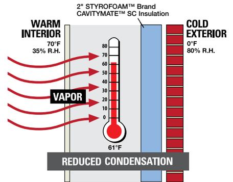
Replacing the batt insulation and exterior gypsum with 2" (50 mm) thick STYROFOAM™ Brand CAVITYMATE™ SC Insulation increases the insulation's interior surface to 61°F (16°C). The cavity is now a conditioned space with the condensation potential near zero. Plus, the system R-value is R-13.1 (RSI 2.31).
