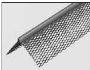
EXPANDED VENEER CORNERBEAD Used as an alternate to the Kal-Korner Bead for exterior corners. 1 1/4" flanges.
