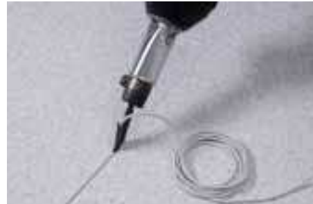
Weld rod seam
