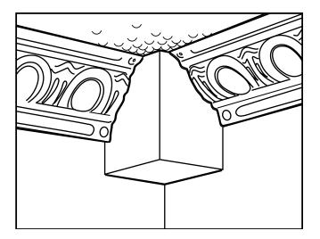
You can also cope inside corners. Butt one piece into the corner. Then trim the second piece on the adjacent wall to fit. First place a strip of masking tape across the end of a scrap piece of molding. Hold the scrap molding in the corner and use a compass or scribing tool to transfer the profile of the nailed-in-place piece to the scrap piece.
