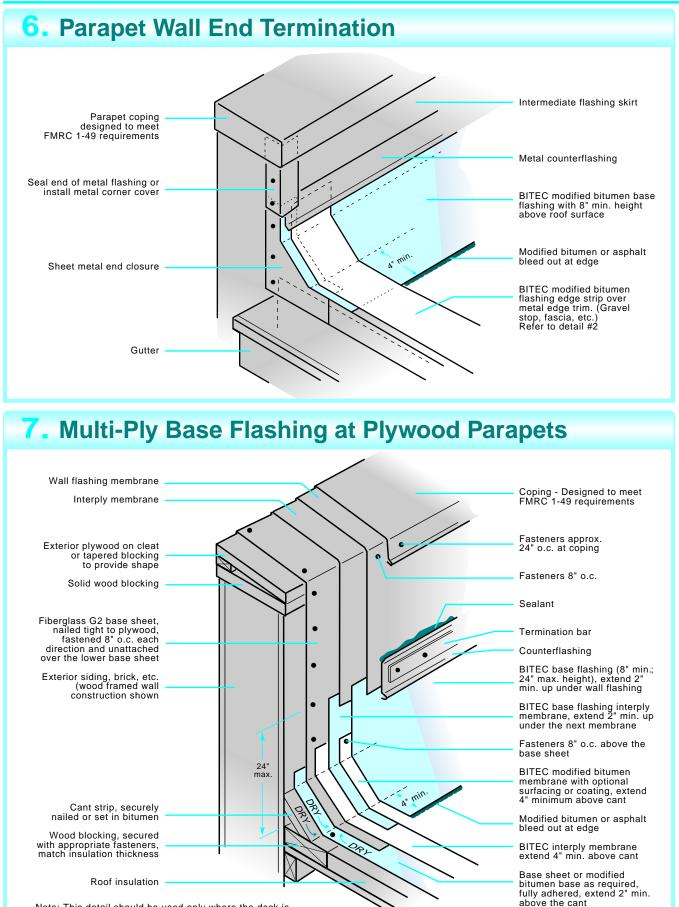
Note: This detail should be used only where the deck is supported by the wall. An expansion joint detail should be used for non wall-supported deck. Contact BITEC Technical Services for suitability of attachment at cants if building movement is not a concern. CONSTRUCTION DETAILS
