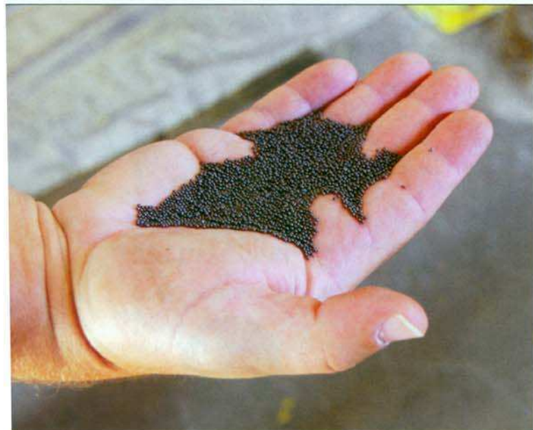
Steel shot (large) is in the rotostator pump and is projected onto the floor at high velocity to smooth it.
