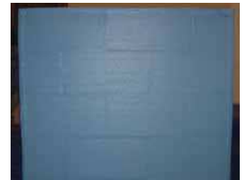
Barritech VP after drying on block. Complete coverage – no pinholes or voids.
