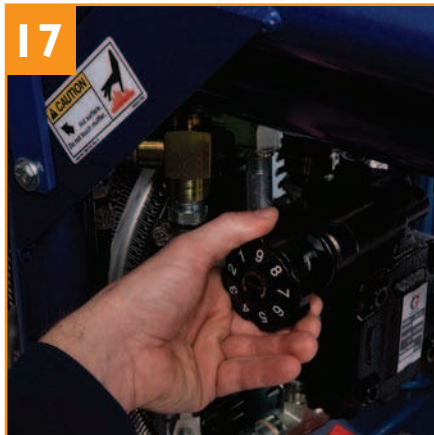
Adjust pressure on Graco pump to initial setting of 1200 psi.
