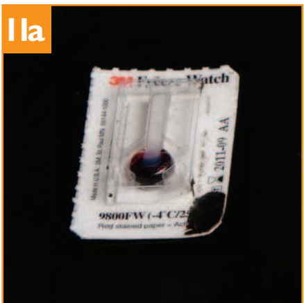
Unbroken freeze indicator If freeze indicator is not broken, proceed to checking the label for shelf life.
