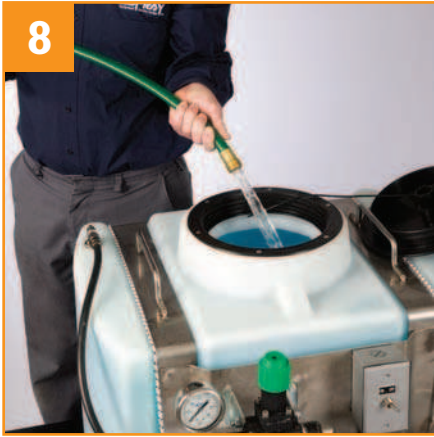
Top off tank on Co-Spray Assembly with clean tap water.
