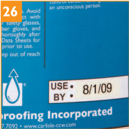
Examine Barritech VP label to determine if material is within shelf life. If material is out of shelf life, call CCW Tech Service.
