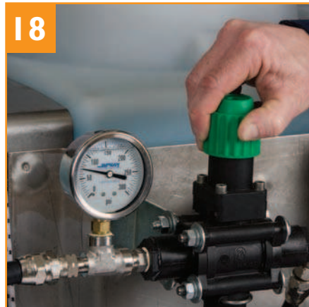
Adjust pressure on co-spray pump to initial setting of 150 psi.
