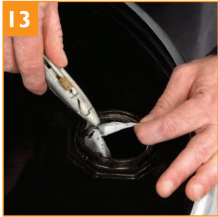
Unscrew bung cap on drum of Barriseal-S or Barricoat-S. Cut membrane that is visible through bung with utility knife.
