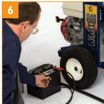
If pump does not have 12 V DC connection, connect clips to 12 V DC generator or 12 V DC battery. (GH 833 Model shown)
