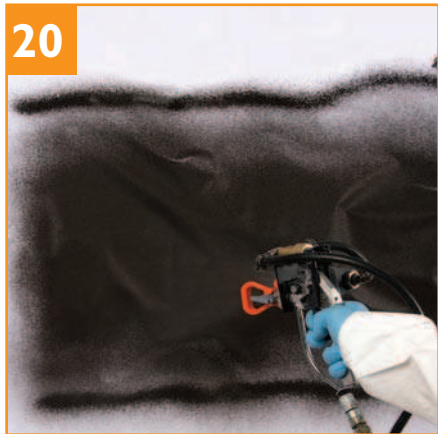
Not Good Uneven spray pattern. Raise pressure or reduce nozzle size to even out spray pattern. Spray must fan out evenly on both Barriseal/Barricoat nozzle and Barricure nozzle. Clean dirty nozzles or replace worn nozzles as necessary.
