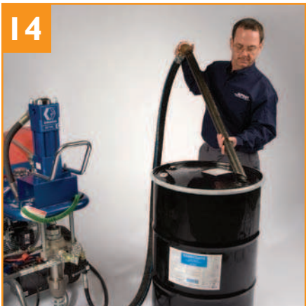
Align intake pipe with larger bung. Set intake pipe all the way to bottom of drum.
