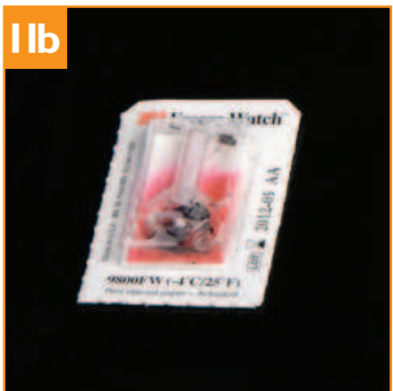
Broken freeze indicator If freeze indicator is broken, shown by red staining, call CCW Tech Service.
