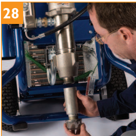
Connect pail adaptor to siphon end of pump.
