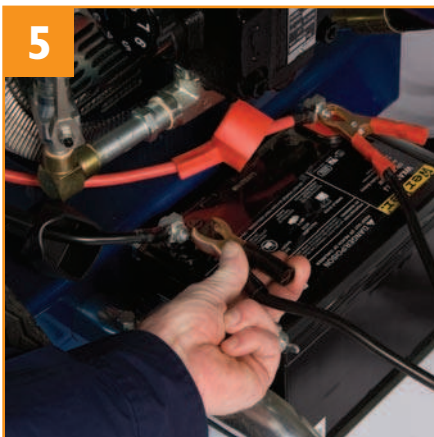
Connect alligator clips to 12 V DC on Graco pump. (GH 733 Model Shown)
