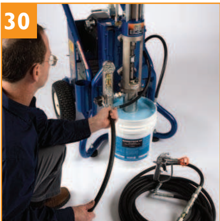
Insert purge line into pail. Connect hose and Graco Silver Gun to discharge of Graco pump.
