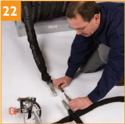
Disconnect gun at quick-disconnect fittings. Disassemble gun and tips, clean Barriseal/Barricoat residue from parts. Thoroughly with citrus cleaner or mineral spirits and reassemble.
