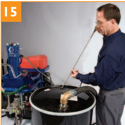
Insert purge wand into smaller bung. Start up Graco pump and adjust settings according to manufacturer's instruction manual.
