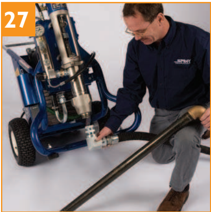
Disconnect drum siphon assembly.
