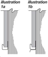
Install the bottom J-channel (illustration 1a). Overlap J-channels 3/4". To do this, cut out a 1" section of the nailing flange and face return (see illustration 2).
