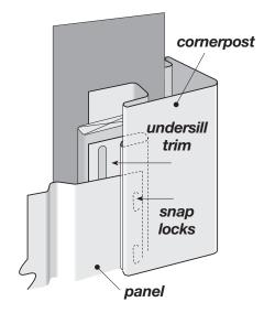
**NOTE:** The cutting and supporting procedure described above is also used when fitting panels into inside cornerposts.
