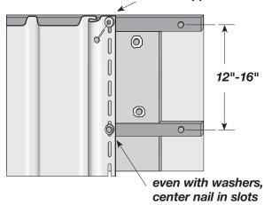
When remodeling over brick, block, stucco or irregular wall surfaces, apply furring strips **horizontally** to create a level surface, then apply rigid foam or fiber sheathing.
