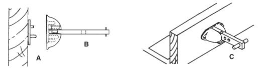
**Removing the Recess Plug from the Concrete:** A) After the back of the recess plug is exposed, insert a steel rod or screwdriver into the half of the recess plug opposite the threaded stud and rotate it to loosen that half of the recess plug. **(B)** After the first half of the recess plug has been loosened, use the holding rod in the other side in a
