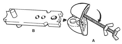
Attaching the Assembly to the Form: A) Place the assembly against the form and position over the predrilled hole. (B) Insert the 3/8" holding rod through the hole and thread into the recess plug. (C) Pull the assembly tight to the form by firmly tightening the wing nut on the holding rod.
