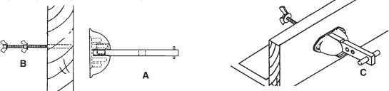
Attachment Using a Holding Plate: A) Position and attach the holding plate to the form. B) Slide the anchor assembly over the holding plate studs and firmly against the form. (C) Installation is complete.
