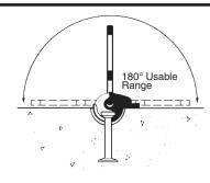
The bail of the P-50 lifting eye can move through a 180° usable range.
