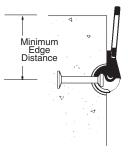
The main body of the lifting eye has a 360° rotational range.
