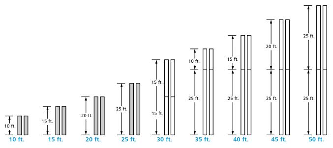
some methods of attaining the various lengths of strongbacks are illustrated below.
