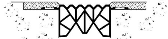
THERMAFLEX is constructed of extruded thermoplastic Santoprene® rubber sealing glands with punched flanges embedded in a high-strength, flexible, impact-absorbing elastomeric nosing.
