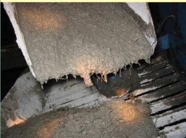
These synthetic structural fibers are a patented, coarse monofilament, self-fibrilating polypropolene/polyethylene blend, successfully used to replace welded wire mesh and steel fibers in a wide variety of applications. TUF-STRAND SF fibers are designed to provide shotcrete with increased flexural toughness, impact and fatigue resistance with the added benefit of superior plastic shrinkage cracking control.
