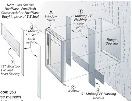
*Note:* You can use *Moistop neXT* in place of *Moistop PF* in base flashing applications.
