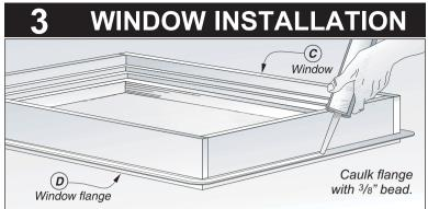
Before installing the window (C), apply a continuous <sup>3</sup>/8" bead of **Moistop Sealant** to the perimeter of the rough opening or to the backside of the mounting flange (D) of the window. Install the window according to the window manufacturer's instructions.
