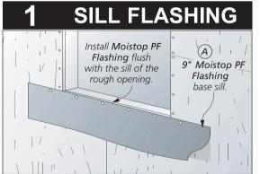
Once the rough opening is prepared, proceed by attaching **Moistop PF Flashing (A)** flush along the bottom of the rough opening extending the flashing beyond the jamb flashing to be applied later. Be sure not to fasten the lower edge of the flashing so that a Fortifiber weatherresistive barrier may be slipped up underneath the flashing in a weather-board fashion.
