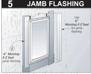
Using a sharp knife, cut the desired length of **Moistop E-Z Seal** for the jamb (**E**) of the window, extending beyond the flange (3" minimum top and bottom). Place the **Moistop E-Z Seal** on top of the flange (**D**) and seal by applying pressure along the strip. Repeat for the other jamb.
