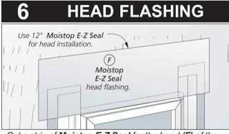
Cut a strip of **Moistop E-Z Seal** for the head **(F)** of the window extending beyond the jamb flashing already in place. Place the **Moistop E-Z Seal** on top of the flange **(D)** of the window with the adhesive strip overlaying the flange and seal by applying pressure along the strip. If desired, staples or sealant may be used to secure the top corners of the head flashing in place.
