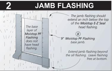
Cut a strip of **Moistop PF Flashing** long enough to extend beyond sill flashing already in place and above where the **Moistop E-Z Seal** head flashing will intersect. Next, attach the jamb flashing (B) flush to the edge of the rough opening leaving the bottom free. Repeat above steps for the remaining jamb.
