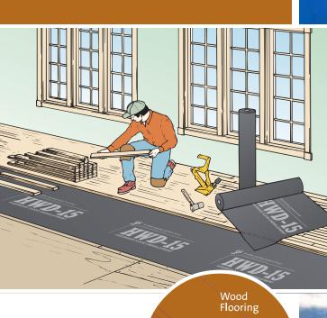
HWD-15 hardwood floor underlayment is an economical and extremely effective Class III moisture vapor retarder specifically designed for optimum performance in wood flooring applications. Consisting of a single layer of kraft paper saturated with asphalt, HWD-15 is a permeable vapor retarder. It reduces vapor flow, without trapping moisture.
