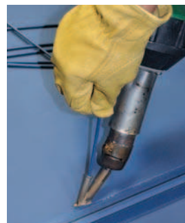
Step 4 - Permanently weld with SecureRod™
