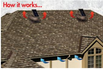
Hot, stale attic air is removed through the solar-powered roof exhaust vents. Fresh air is drawn into your attic through you soffit (or other) intake vents.
