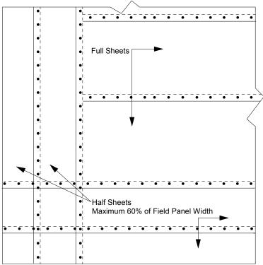
All GenFlex TPO Mechanically Attached Systems require half sheet perimeter securement. A half sheet width of up to 60% of the width of the field panels may be used. Half sheet securement is equal to the membrane securement used in the field of the roof. See the Mechanically Attached TPO Fastening Matrix for fastener and spacing requirements. If the project must meet Factory Mutual criteria, refer to Detail T-42.04-3, and contact Factory Mutual for review.
