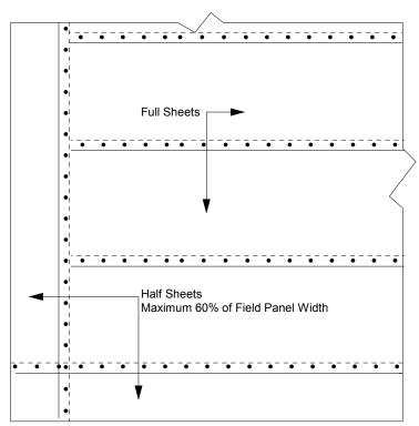
All GenFlex TPO Mechanically Attached Systems require half sheet perimeter securement. A half sheet width of up to 60% of the width of the field panels may be used. Half sheet securement is equal to the membrane securement used in the field of the roof. See the Mechanically Attached TPO Fastener Matrix for fastener and spacing requirements. If the project must meet Factory Mutual criteria, refer to Detail T-42.04-3, and contact Factory Mutual for review.
