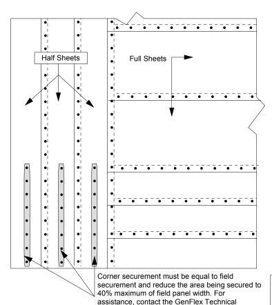
As an option, corner enhancement may be accomplished by installing additional rows of securement through the half sheets and then stripping-in those rows of securement with GenFlex TPO Cover Tape after first applying GenFlex Clear Primer with a Scrub Pad & Handle.
