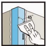
◆ Tip: When applying NO-COAT° corners, embed trim by running a 4-6" taping knife over it with even pressure at a 45° angle. Wet compound should ooze out past the paper flap.
