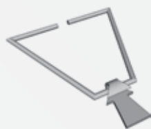
#103 Dovetail Triangular Tie: 12 gage clip with 3/16" dia. wire tie. For Brick and CMU.
