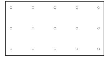
Fasteners must be installed at all panel corners and at a maximum of 24" o.c. in both directions throughout the entire panel surface. In panels where a splice occurs, additional fasteners must be installed on both sides of splice at a maximum of 6" from splice and 24" o.c. Fasteners must be held back 1 1/2" from edge of panel. 1-90 Classification is achieved without roofing plates.
