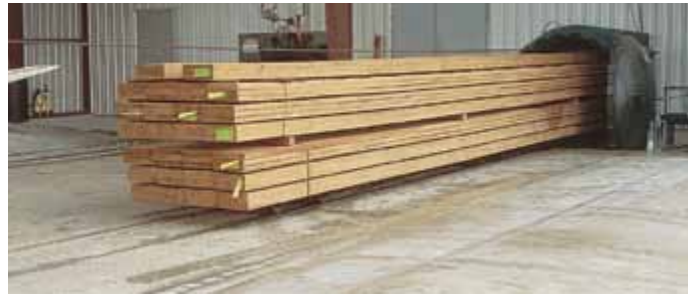
Parallam® PSL products enter an airtight treatment cylinder—a highly controlled, pressurized environment where they are exposed to the Wolman® treatment process.
