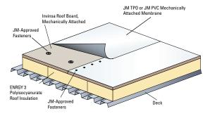
Mechanically fastened, JMTPO or JM PVC single ply roofing system. For use over JM-approved decks or other approved insulation.
