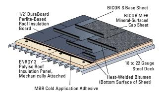
Two-ply, heat-welded, modified bitumen, mineral-surfaced roofing system. For use over JM insulation, approved decks or other approved insulations on inclines up to 6 inches per foot (500 mm/m).
