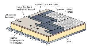
Two-ply, modified bitumen, roofing system with a self-adhering base sheet and heat-welded cap (2FID SA/HW). For use over JM insulation, approved decks or other approved insulations on inclines up to 3 inches/foot (250 mm/m).
