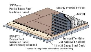
Four-ply, gravel-surfaced, fiber glass built-up roof. For use over JM insulation, approved decks or other approved insulations, on inclines up to 3 inches per foot (250 mm/m).
