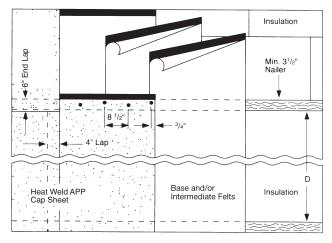
**7A.22.5** Nailable and Lightweight Concrete Decks: On decks with a slope over  $1\frac{1}{2}$ " per foot (125 mm/m), the roofing felts must be installed parallel to the incline. Nail the end laps of the modified bitumen cap sheet across the width of the sheet on  $8\frac{1}{2}$ " (216 mm) centers. All nails are to be covered by the lap of the next sheet.
