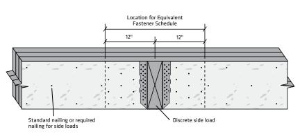
**EXAMPLE:** Assuming a properly designed 3-ply 14" beam, determine the equivalent connection to support a 3300 lb point load applied to the side of the beam.
