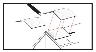
Starter: cut the 5%" exposed portion of a Hip & Ridge Strip. Use the remainder (7%") portion as a starter. Fasten approximately 3" in from roof edge. Lay first full Hip & Ridge Strip even with ridge starter shingle. Use two nails per shingle, with one nail on each side approximately 1" (25 mm) in from
