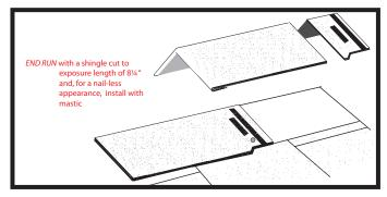
At last shingle in the run, remove the cutout end of an EZ-Ridge shingle and trim to fit maintaining the 8 ¼" (209.5mm) exposure. Set shingle in mastic.
