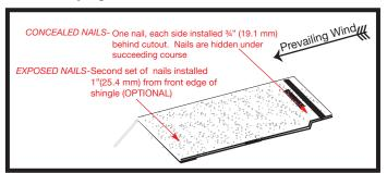
Concealed Nails: Install one (1) nail on each side of the hip & ridge shingle ¾" behind the cut out (not on the exposed part of the shingle). Use a ¾" head non-corrosive roofing nail, long enough to penetrate all layers and attach the shingle to the roof deck.
