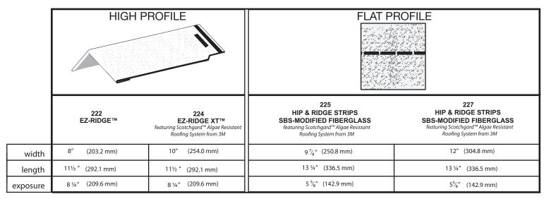
ALL MALARKEY HIP AND RIDGE SHINGLES INCLUDE A FACTORY-APPLIED, THERMALLY ACTIVATED SEAL DOWN ADHESIVE THAT PROVIDES ADDITIONAL PROTECTION AGAINST BLOW OFF.
