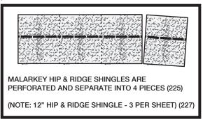
Apply Malarkey Hip and Ridge shingles beginning at bottom of the hip or from the end of the ridge opposite the direction of the prevailing winds.
