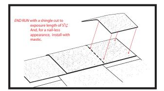
Trim the seal down end of a Hip & Ridge Strip to fit at end, maintaining the exposure length of 5%" (149.2mm). Set shingle in mastic.
