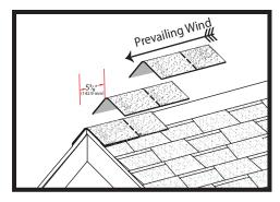
Continue installing ridge shingle with a maximum exposure of 5%" and fastening with one (1) nail on each side, 1" (25 mm) in from each edge. Nail placement will allow for concealment of nail head with next course.
