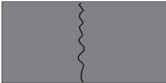
Cracking of Irregular Panels
