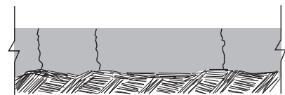
Uneven Grade Can Cause Cracking
