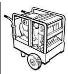
Stable Power* 110–125 volts, 60 Hz *Use 5,000 watt (min.) generator with one 20A GFCI protected circuit per tool. Two tools per 5,000 watt generator.
