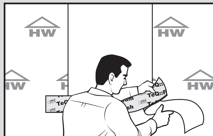
(Figure 2) Sill flashing installation.
