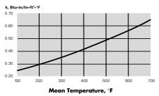
Apparent thermal conductivity curve determined in accordance with ASTM Practice C 1045 with data obtained by ASTM Test Method C 335. Values are nominal, subject to normal testing and manufacturing tolerances.
