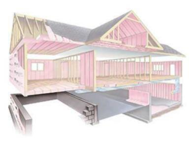
FOAMULAR® rigid foam insulation installs directly against your foundation wall from the footing to the top of the grade. It offers excellent moisture resistance so it won't lose any insulating power (R-value) even after long-term exposure to wet soil and ponding water. Its rugged construction readily withstands the pressure of backfilling and resists the effects of acids and other decaying elements in the soil.
