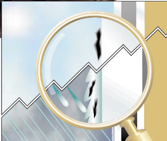
The photocatalytic action of Pilkington Activ™ Glass ( upper ) gradually breaks down and loosens dirt, while the hydrophilic surface ( lower ) causes rain to sheet on the glass, leaving a clean exterior surface with minimal spotting or streaking. (Illustration shows cross-section of glass I.G. unit. Outboard lite is shown magnified to demonstrate the effect of the Activ™ Glass surface.)
