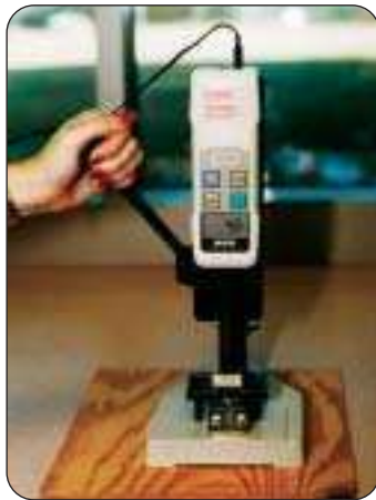
Cross-Axial chisel split test – A digital force gauge measures the applied load in testing small cores.
