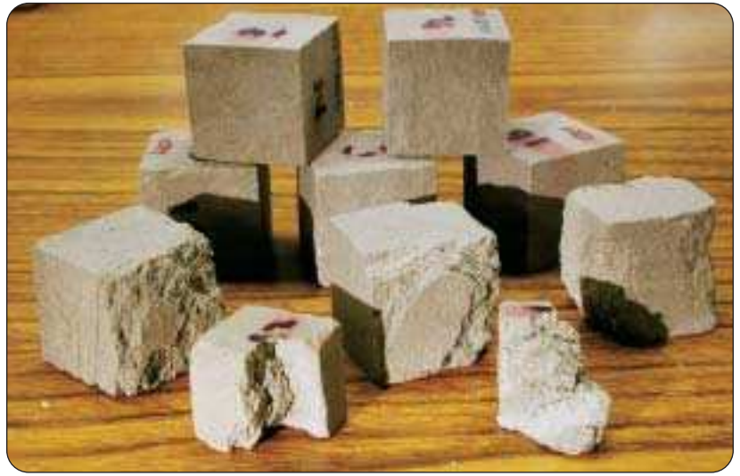
Freeze/Thaw resistance – Treated cubes (background) and untreated cubes (foreground), after 29 cycles of freezing and thawing.
