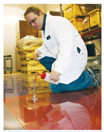
**Fig. 3 - Rilem Tube Test:** Consolideck® professionals are trained in the use of standardized performance tests. Here, a technician uses the kit's Rilem Tube to check the water-resistance of a Consolideck® Decorative Performance Floor.
