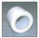
Canvex Seal Tape is a single-sided white woven tape that contains an acrylic adhesive with a release liner. It has excellent adhesion to polyethylene and the acrylic adhesive provides much longer life than many competitive tapes. It is recommended for taping the seams on in-wall vapor retarders and crawl spaces. Available in a 4" x 100' roll.
