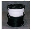
Raven Welding Rod is used for field seaming, repairs and detail work, such as installing pipe boots. Packaged in 10 lb spools, it is available in 4mm and 5mm sizes to fit most brands of extrusion guns. Raven Welding Rod is made from a thermally UV stabilized LLDPE resin and is available in both black and white to correspond with the color of geomembranes being utilized.
