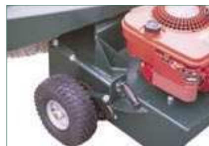
Adjusts to sweep left, right or straight ahead
