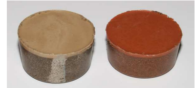
Roadware MatchCrete Concrete Mender™ with sand on the left and with sand and Solomon brand color on the right.
