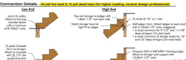
NOTE: Only use fasteners approved for use with the corresponding wood treatment.
