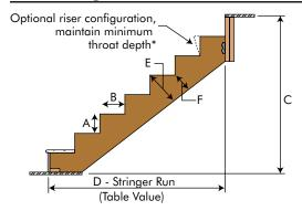
A - Step Rise: Vertical rise of a single step B - Step Run: Horizontal length of a single step C - Total Rise: Vertical distance from top of finished framing on low end to
