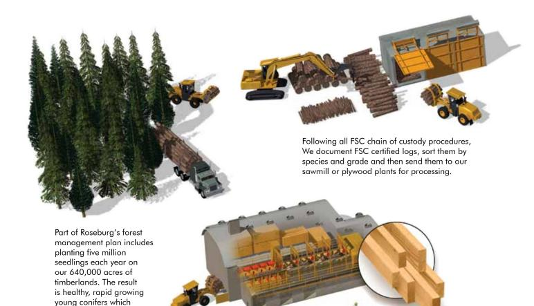
of lumber at our state-of-the-art sawmill is sorted and sent to either the composite panel plant to make particleboard or the biomass cogeneration plant to create energy for the facilities and local communities.
