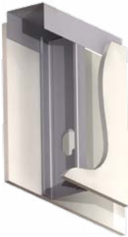
Fully sheathed with no additional bracing
