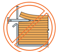
Nail at wrong angle
