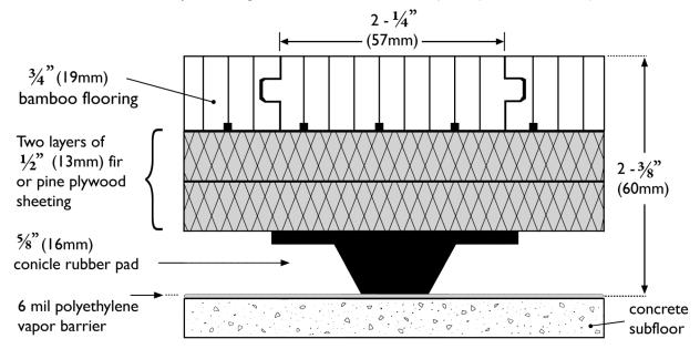
A. End View Detail: System Diagram with CenterLine starter plank (3/4" x 2 1/4" x 72"):
