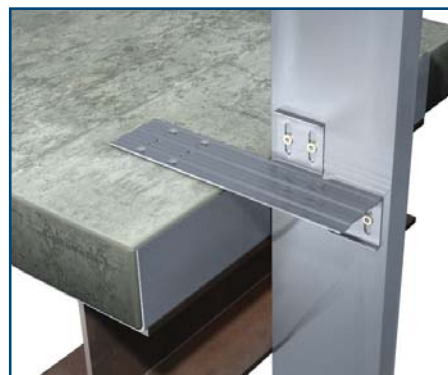
Align studs to SLT for plumb wall assembly.
