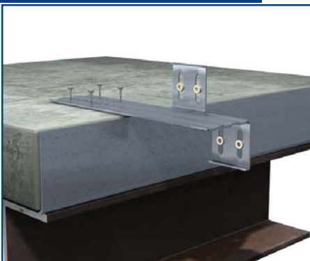
Attach SLT to top of slab with engineered attachment. Allow 4" minimum clip area for attachment to slab.
