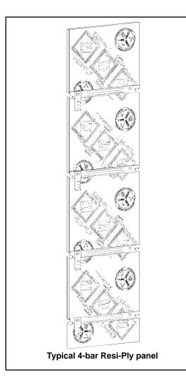
The Resi-Ply forming system is a 1½" thick plywood with steel backing bars designed especially for residential foundations and low industrial concrete walls.
