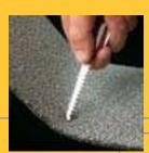
**TAKE A STAB AT US.** Use one of the blunt-ended tools on your pocket knife and try to puncture roofing samples. Inferior products will puncture and crack. But the unsurpassed strength of the polyester mat allows Awaplan membranes to demonstrate a much higher puncture resistance.
