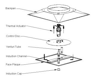
The thermal T<sub>3</sub>SQ uses a center mounted induction cap to accurately measure the room temperature. This eliminates the need for a wall mounted thermostat or sensor and provides the fastest, most accurate way of measuring the room air temperature.
