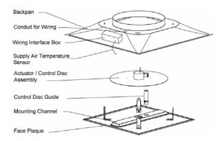
Master diffusers are created by connecting the  $T_3SQ$ -1 diffuser to a wall mounted controller / thermostat using the blue RJ-45 control cable.  $T_3SQ$ -1 drone diffusers are created by connecting the diffuser to a master unit using the blue RJ-45 control cable.
